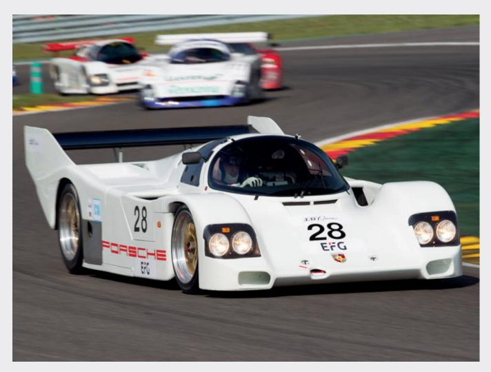
From this starting point Porsche not only stretched the wheelbase but also implemented their famous **PDK gearbox** as well as optimise their fl at six turbo engine. The much used and highly efficient ground effect which was first developed in the **956** was carried over to the **962C** with great success.
