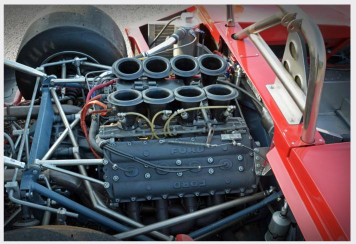
To handle the enormous power and torque of the DFV engine, a Hewland FG400 gear-box, new shocks and springs, ventilated disc brakes and Lockheed brake calipers were fitted, while the bodywork was enlarged to make room for the new 15-inch wheels.
